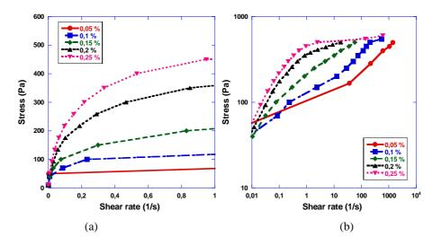
*Figure 5.* Flow curves obtained in the stress-controlled mode using different polymer contents. (a) Linear plot (for lower shear rate values). (b) Logarithmic representation (for higher shear rate values).
