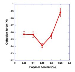
Figure 3. Evolution of the cohesion force with polymer content.
